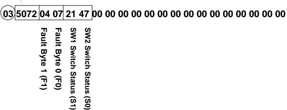
Slot 3 shows that the Fault status is 0407 (F1, F0). The Status report read-out is 2147(S1,S0).
